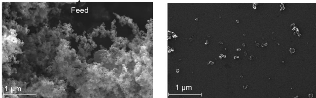
SEM images: feed material carbon black (left); after dispersing in water (CTAB) in a batch mill (right)
