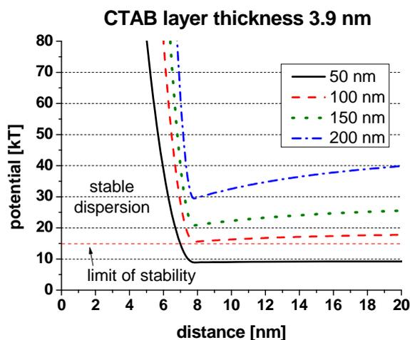
Extended DLVO calculations (carbon black particles + CTAB): smaller particle diameter → smaller repulsion → instability (potential < 15kT)
